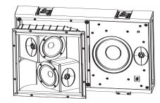
Figure 13. Rotate top baffle for vertical or horizontal orientation
